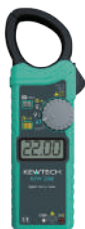
KYORITSU 2200 AC A : 40/400/1000A AC V : 4.000/40.00/400.0/600V DC V : 400.0mV/4.000/40.00/400.0/600V \Omega : 40.00M \Omega Hz : 4 kHz Jaw Opening : \varnothing 33mm CAT III - 1000V CAT IV - 600V
