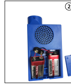
Ensure placement is matching battery (+ positive & - negative)
